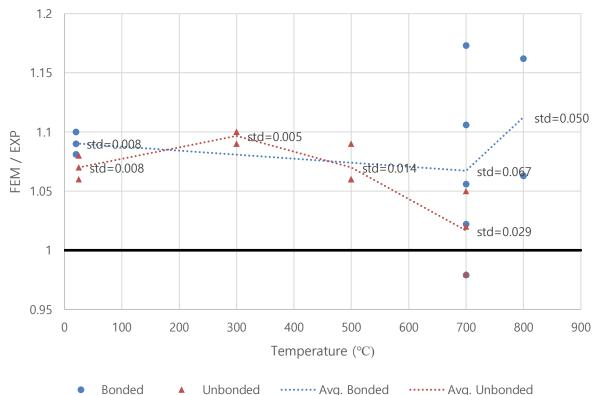
Fig. 1 Comparison of ultimate loads of concrete beams obtained from FEM analysis and experimental tests at different temperatures
